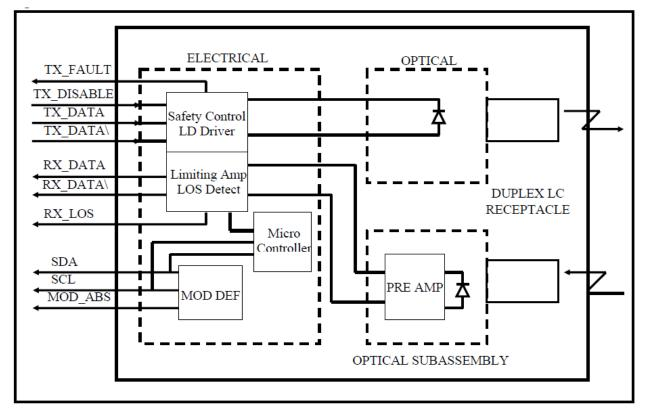
**Transmitter Section-** The Laser driver accept differential input data and provide bias and modulation currents for driving a laser. An automatic power-control (APC) feedback loop is incorporated to maintain a constant average optical power. 1330 DFB in an eye safe optical subassembly (OSA) mates to the fiber cable.
